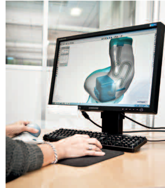
Figure 5. The sound bore is folded optimally for the individual client's ear canal.
