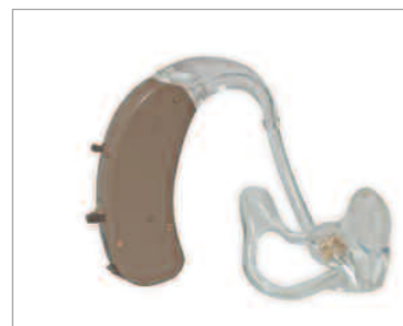
Figure 1. The long tubing of a traditional BTE increases the output by amplifying the sound that travels through it.
